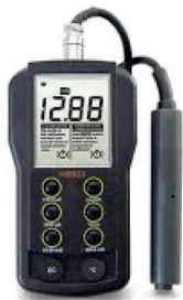
Measurement device for measuring conductivity, pH values and the temperature of the fountain solution
